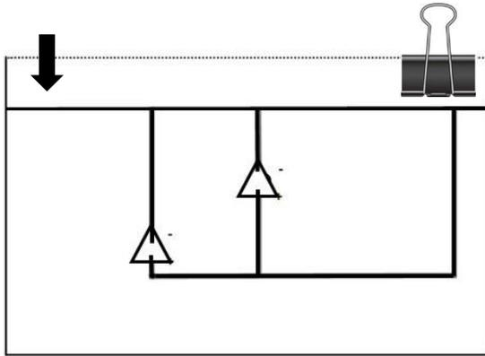
Crease along the FOLD line along the top so that the two circles are on top of one another. Place the battery within the fold with the positive side down on the paper. Make sure the copper foil tape is touching the battery on both the positive and negative side. Hold the battery in place using the paper or binder clip.
